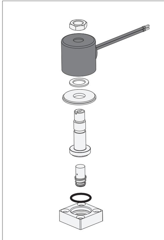
Figure 4. 40M Valve, Exploded View
