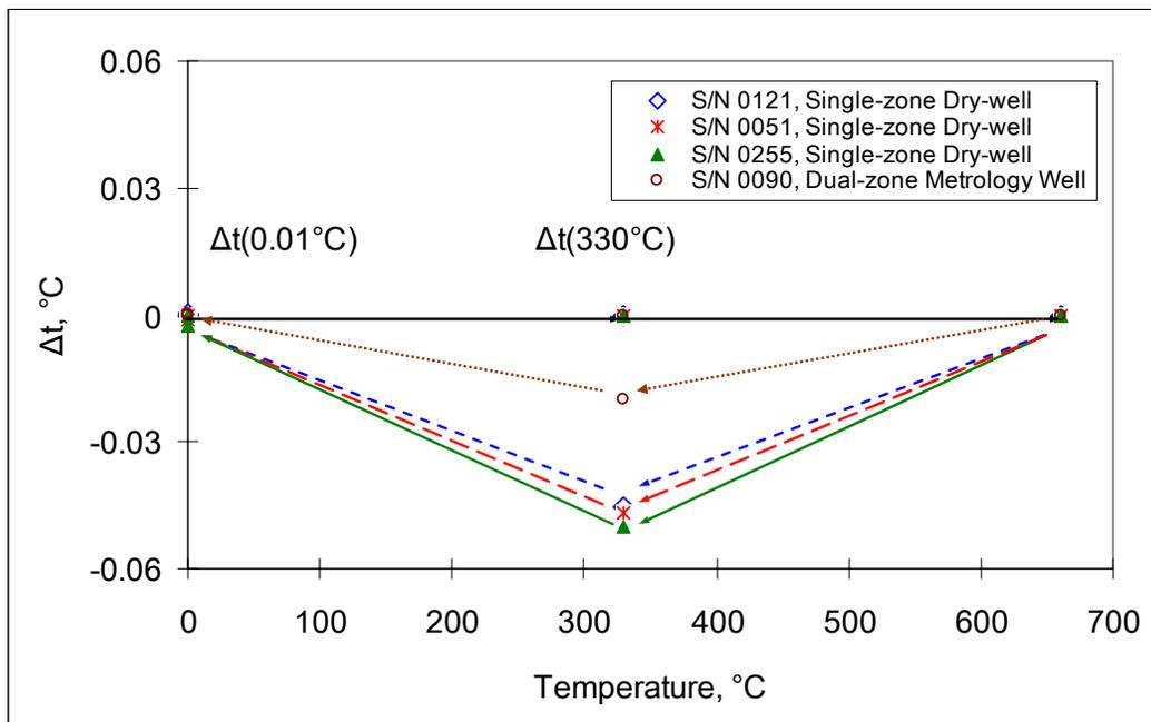
Figure 6, Effect of Hysteresis of the Control Sensor
