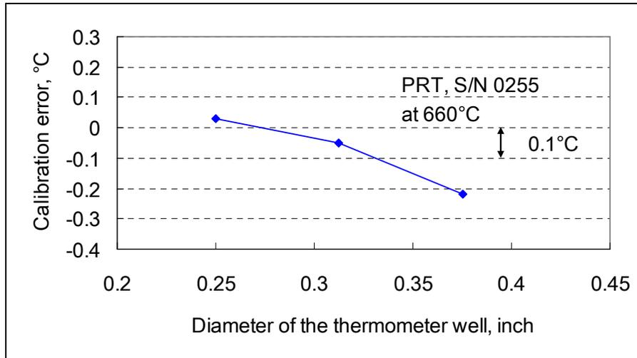
Figure 8, Measurement errors when the diameter of the PRT does not match the well diameter
