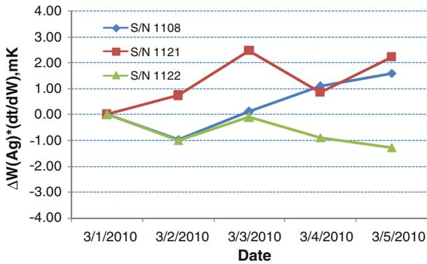
**Fig. 6** Short-term stability at the freezing point of silver
