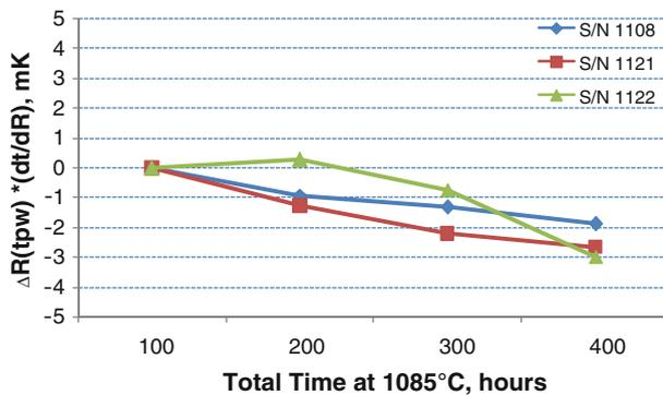
**Fig. 3** Long-term stability at the triple point of water
