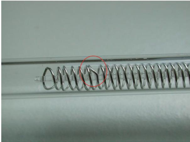
**Fig. 1** Short circuit of HTSPRT sensor with strip support
