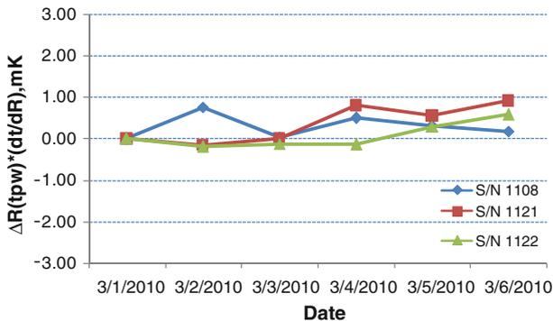
**Fig. 5** Short-term stability at the triple point of water
