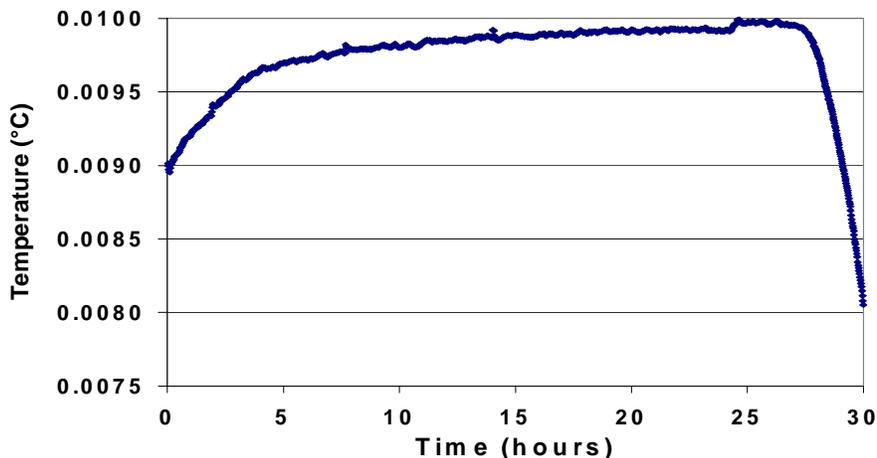
Figure 3. A typical freezing curve in a mini TPW cell
