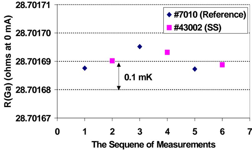
Figure 7. A direct comparison of a SS Ga cell #43002 with Hart reference Ga cell #7010
