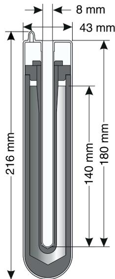
Figure 9. A small-size fused silica-cased fixed-point cell
