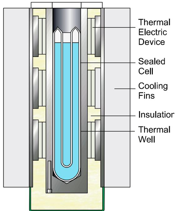
Figure 2. A portable semi-automated apparatus for realizing the TPW using a mini cell
