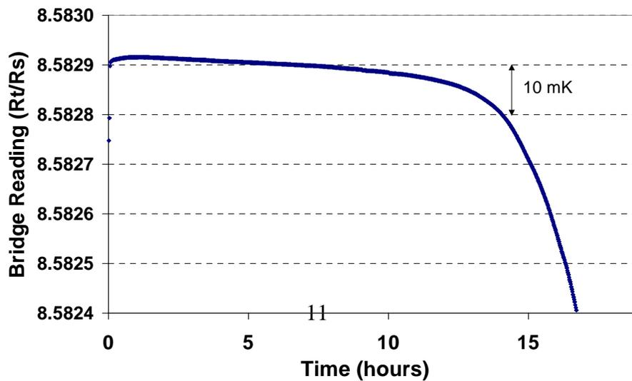
Figure 13. A freezing curve of aluminum, using a small-size cell
