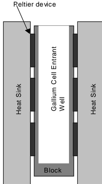
Figure 6. Cut away view of the automatic gallium apparatus
