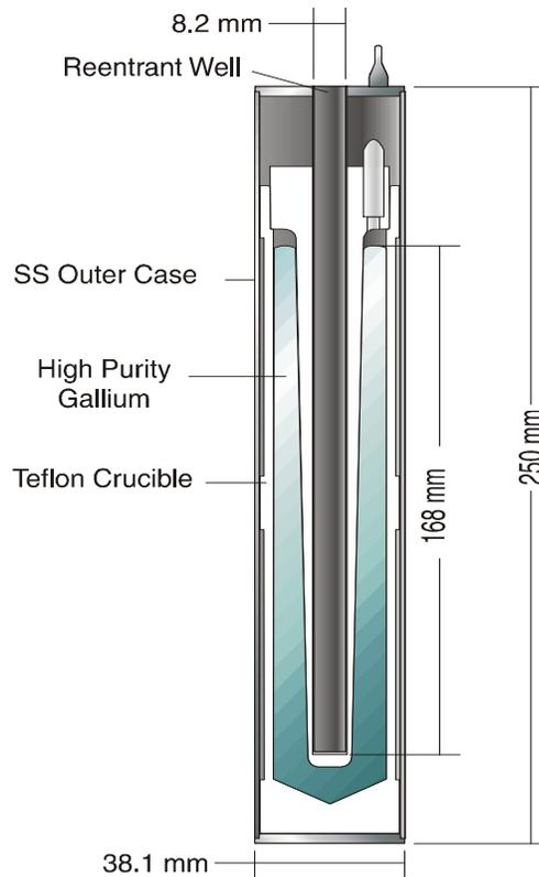
Figure 5. Schematic diagram of the new MPG cell
