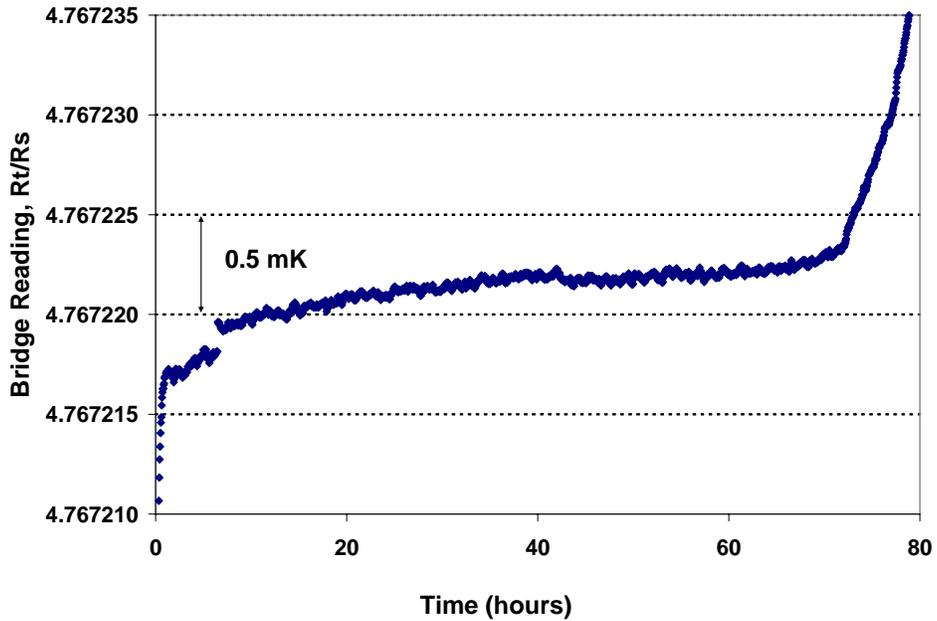
Figure 12. A melting curve of tin, using a small-size cell
