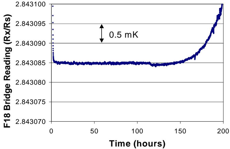
Figure 8. A typical melting curve using the new SS cell and automatic maintenance apparatus
