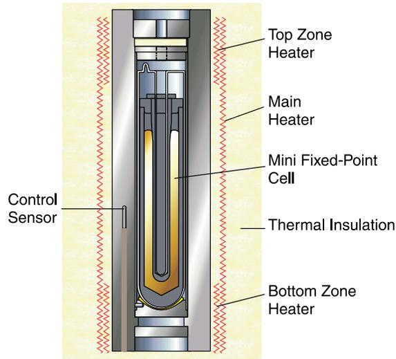
Fig. 11. A small-size fused silica-cased fixed-point cell in a portable furnace
