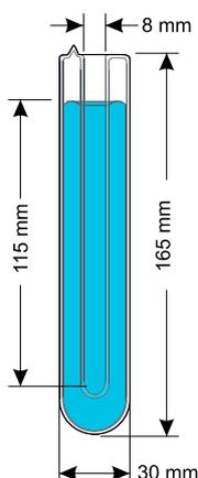
Figure 2. A portable automated apparatus for realizing the TPW, using a mini cell.
