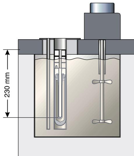
A number of freezing and melting curves were obtained using mini cells. Figure 12 shows a melting curve of tin in a salt bath. Similar baths are commonly found in many secondary laboratories. The melting plateau lasted for more than 75 hours and the change in temperature during 92% of the plateau was within 0.6 mK. Many thermometers can therefore be calibrated during a single melting plateau. A freezing curve of aluminum, obtained in a portable furnace, is shown in Figure 13.
