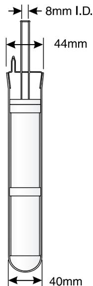
Figure 6. The sealed gallium cell in a bath
