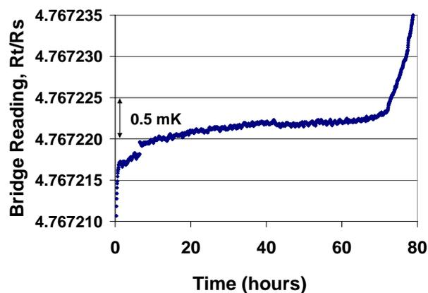
Figure 13. A freezing curve of aluminum, using a mini cell.
