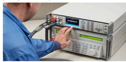
The capacitance traceability for the transfer standard is derived from voltage, current and time which has been validated against reference capacitors and a standalone measurement system which is also based on voltage, current and time. This standalone measurement system has been used since the early 90's by Fluke and is listed in the UKAS schedule of accreditation.
