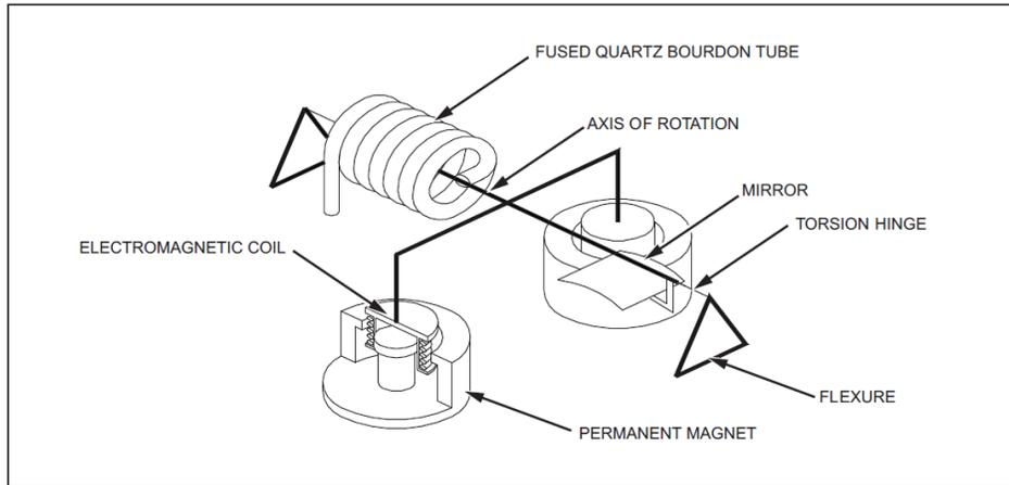
Figure 3. Fluke Quartz Bourdon Tube Sensor Assembly (Drawing).
