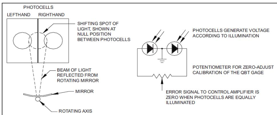
Figure 4. Photodiode Assembly.
