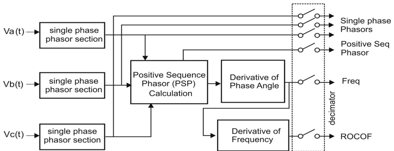
Figure 2. Block diagram of a PMU under test
