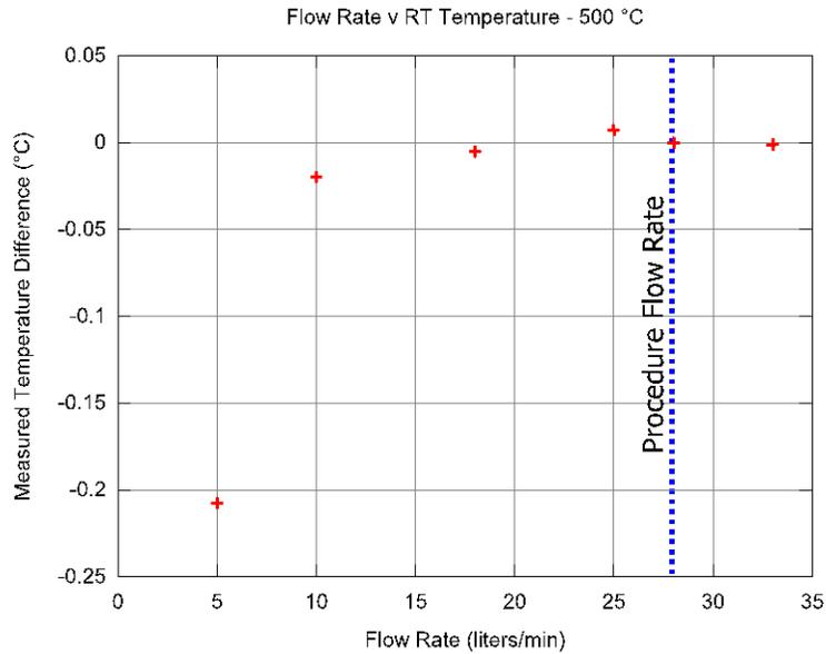
Figure 6. Blackbody purge flow rate test.
