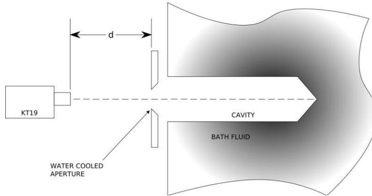
Figure 4. Transfer standard calibration geometry.
