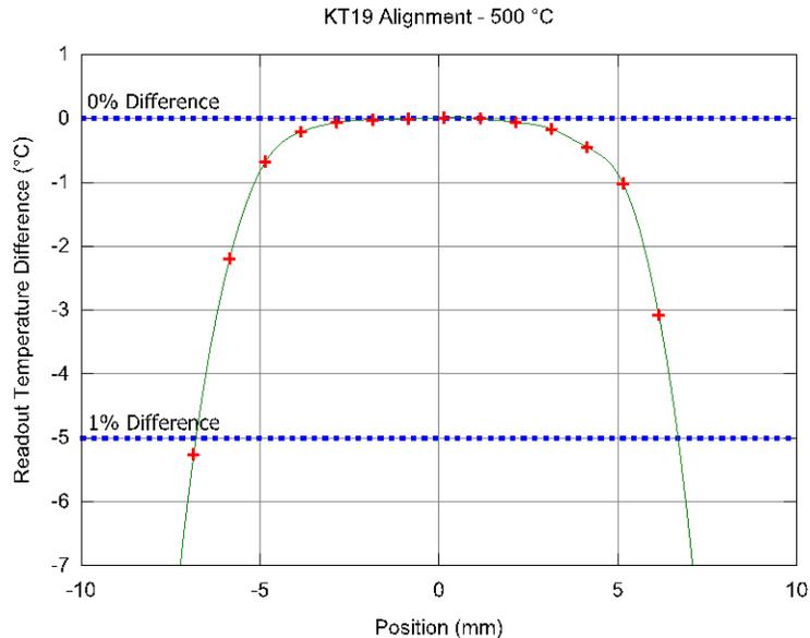
Figure 8. KT19 horizontal alignment.
