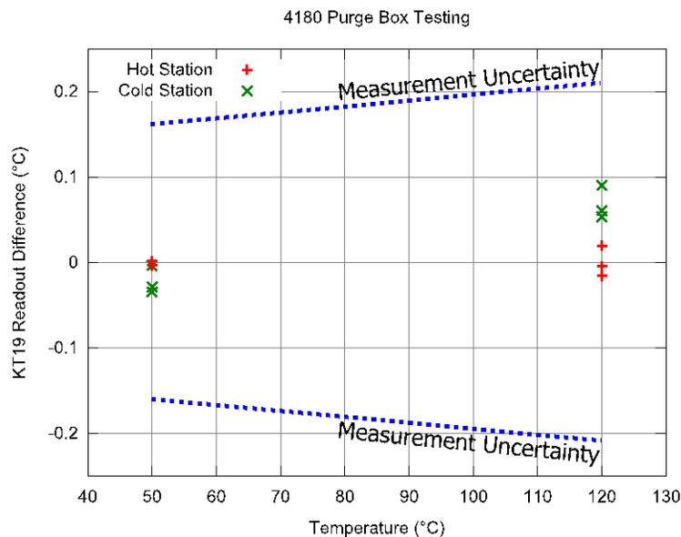
Figure 12. Radiometric measurements with and without purge chamber.
