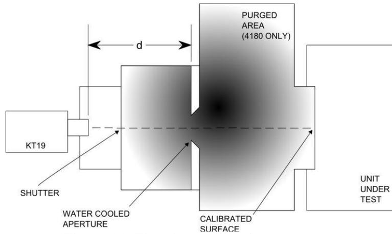
Figure 11. Flat plate calibration geometry.
