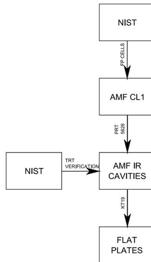
Figure 3. Radiometric traceability scheme
