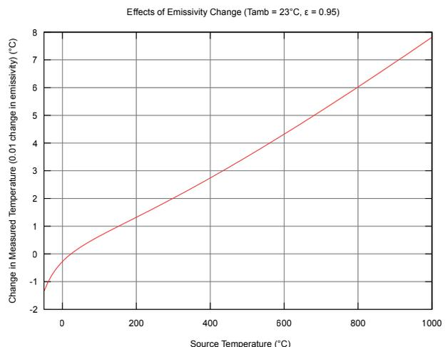
Figure 1. Effect of emissivity error.
