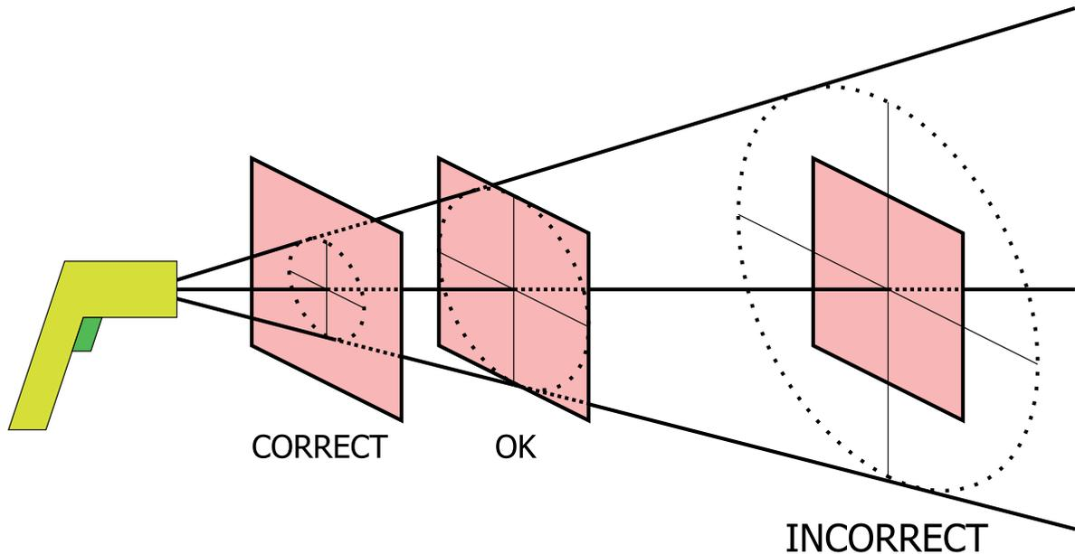
Figure 2. Proper measurement size-of-source.
