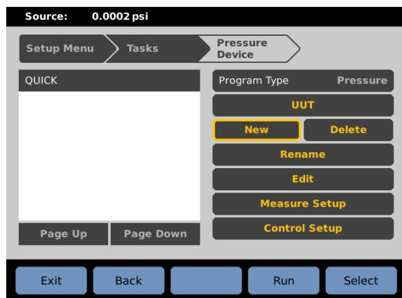
Figure 6. Pressure Device Task Screen with New highlighted
