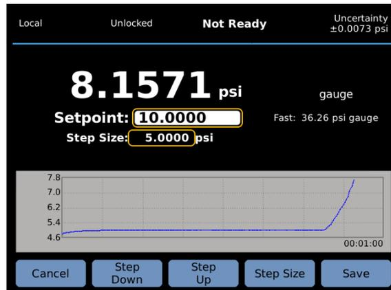
Figure 3. Press Step Up to increase setpoint to 10
