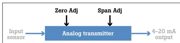
Figure 1. Analog transmitter block diagram
