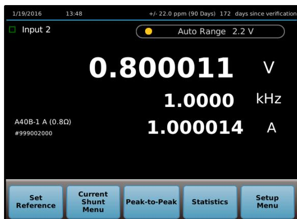
Figure 7. Current measurement
