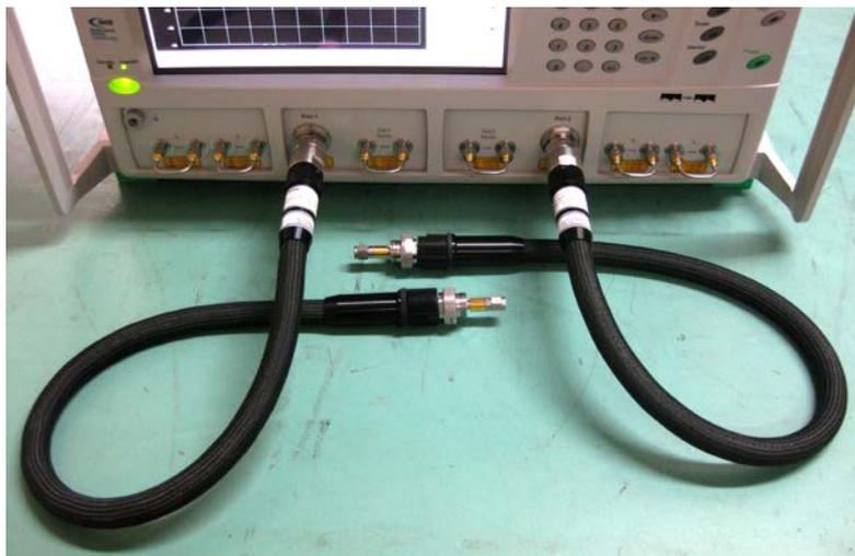
**Figure 4.** Phase and level stable cables used for Vector Network Analyzer (VNA) test port connections.
