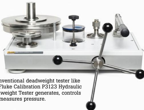
A conventional deadweight tester like this Fluke Calibration P3123 Hydraulic Deadweight Tester generates, controls and measures pressure.
