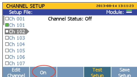
Press the **Edit Channel** soft key, set **Function** to Thermocouple, Thermistor, or PRT. Choose the appropriate parameters for the function selected. Configure additional channels. Press **Back** when finished.
