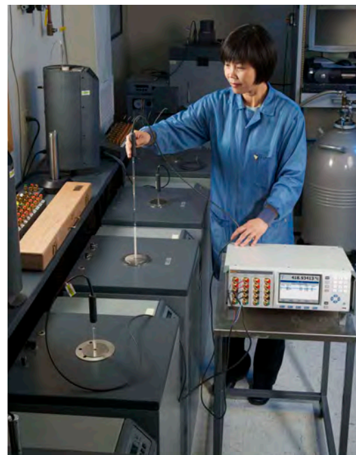
Higher quality ADCs, parallel amplifiers and three isolated power supplies minimize the Super-Thermometer's uncertainty due to measurement noise to 0.02 mK.
