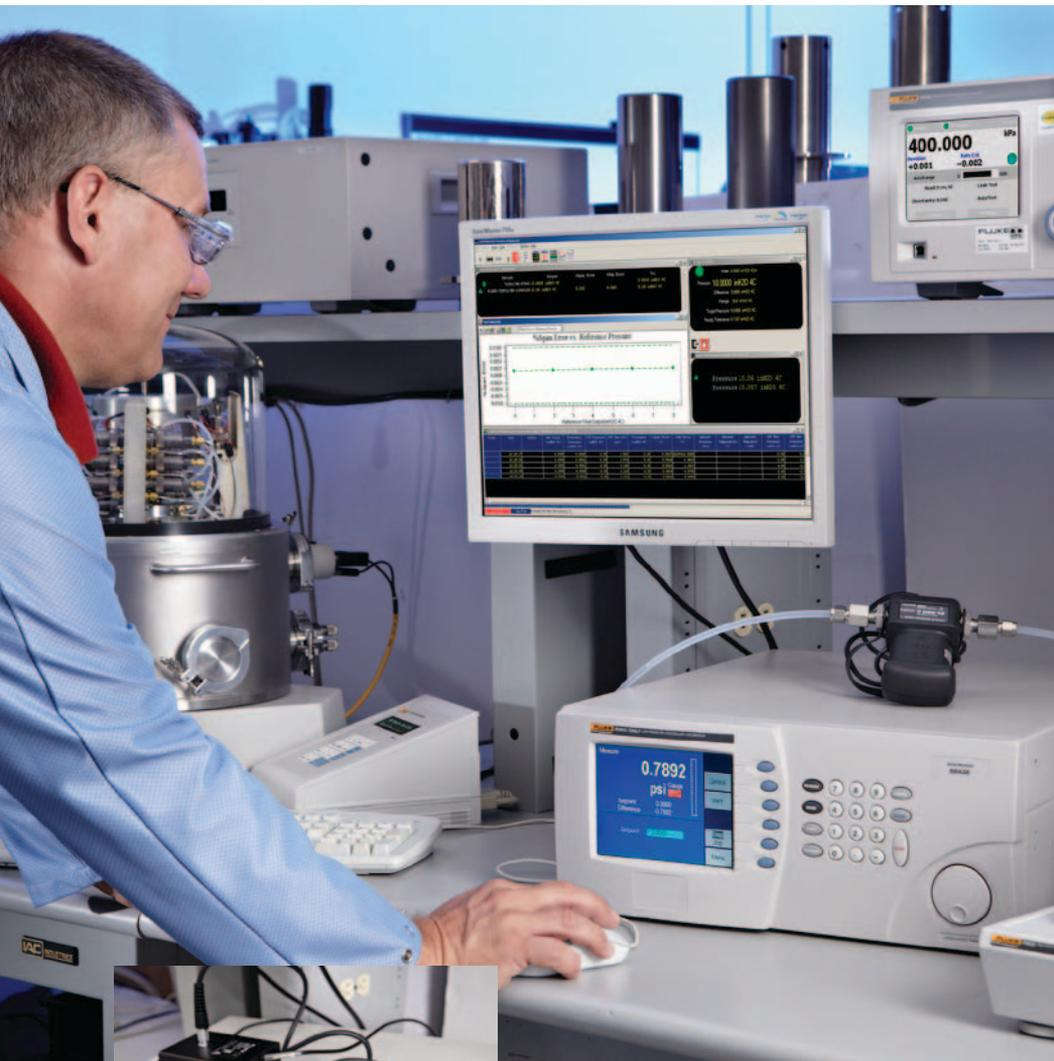
This application note describes how a pressure calibration laboratory can improve throughput by fully automating the calibration of Fluke 700 Series Pressure Modules.
