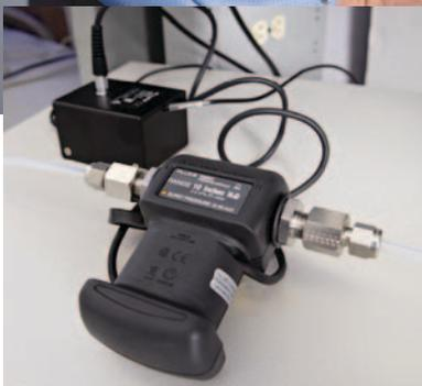
Once the controller stabilized the pressure at the target point, the program would record the pressure value of the controller's reference sensor and also record the value(s) of the instruments being tested. The programs would also communicate with other test hardware necessary for the pressure testing, for example, thermal chambers or programmable power supplies.
