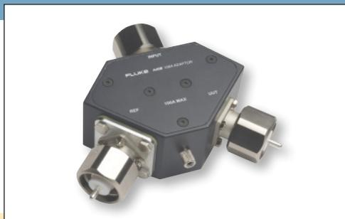
The high current adapter is used when calibrating the A40B shunts at current levels of more than 2 A. It connects together the current source and two shunts for calibration measurements. This adapter uses LC connectors. In this configuration, a certified or reference shunt is connected in series with a shunt that is being calibrated, which in turn are in series with a current source.
