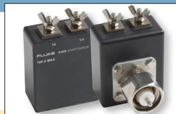
This adapter enables connecting the LC style input connector of the 50A and 100A A40B shunts with sources that use cables equipped with spade lug connectors. This is intended for dc and low frequency ac current measurement applications (up to approximately 1k Hz in frequency).
