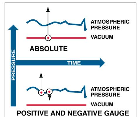
Figure 2. The stability of reference in two common types of the differential pressure.
