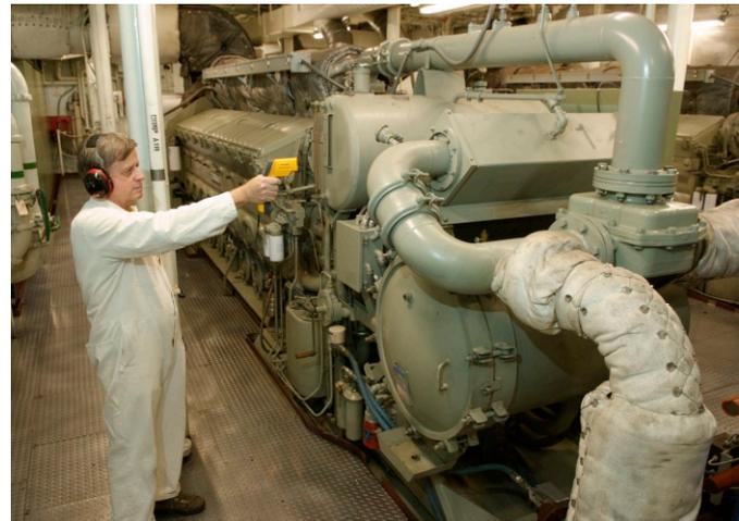
“Every now and again we have sensors go south,” he says, “and I’ll go out and use the IR thermometer for a rationality check to see, we really don’t have 1200 °F on an exhaust section or something like that.” It’s also handy, he adds, “when an RTD goes open and you get infinite temperature.”
