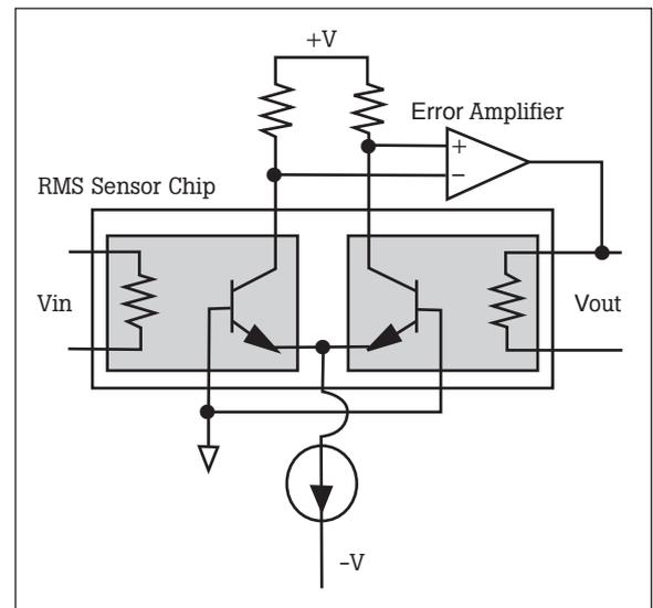
Figure 1. Simplified RMS sensor circuit.
