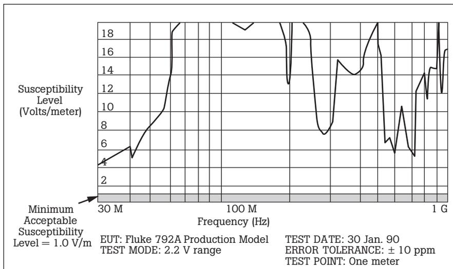
Figure 15. Radiated susceptibility: MIL-T-28800D RS03 (production model).
