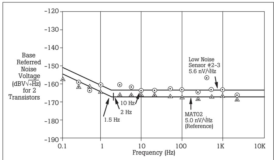
Figure 3. Base referred voltage noise: improved sensor.
