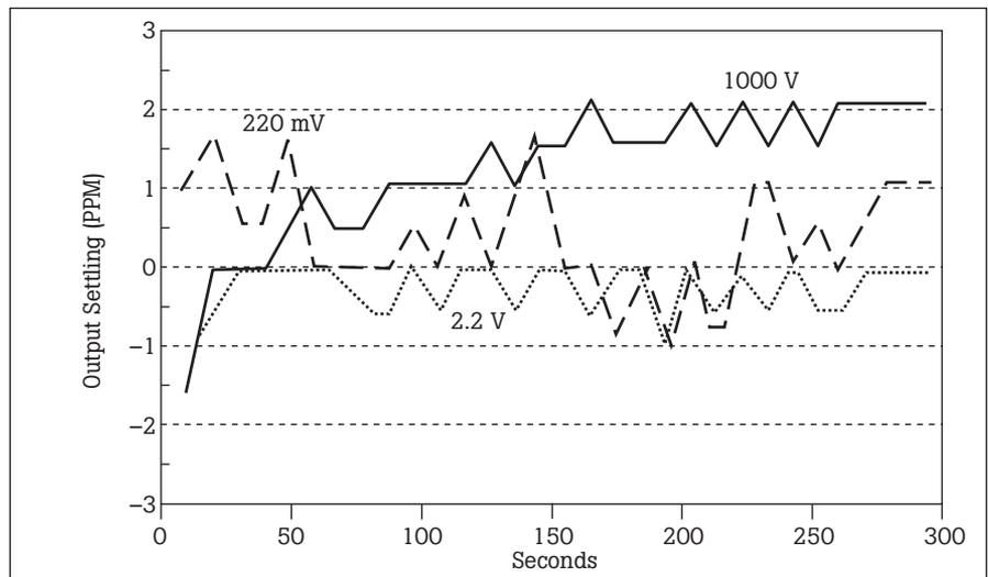
Figure 12. 792A output settling: 220 mV, 2 V ranges.
