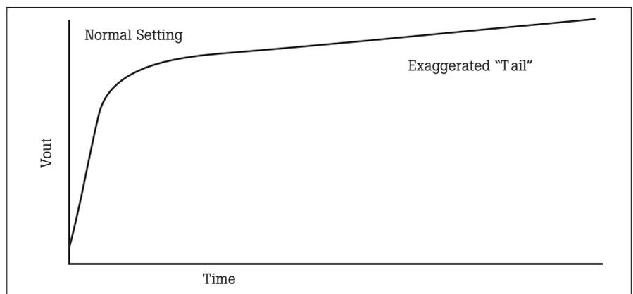
Figure 4. RMS sensor output settling before thermal improvements.
