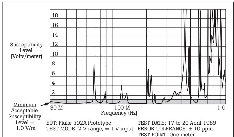
Figure 14. Radiated Susceptibility: MIL-T-28800D RS03 (Design Model).
