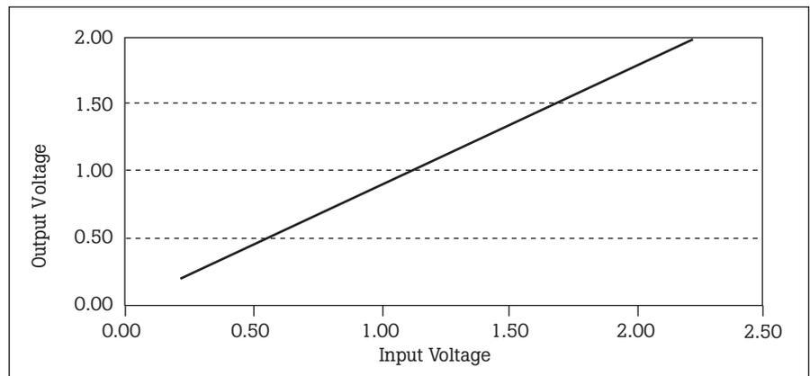
Figure 8. Linearity of 792A 2 V range: 0.22 to 2.2 Volts.
