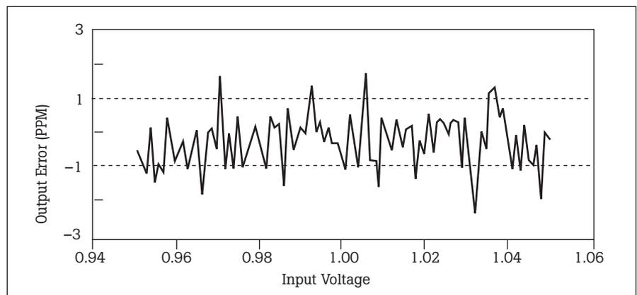
Figure 9. Linearity error in 792A 2 V range: 0.95 to 1.05 Volts.
