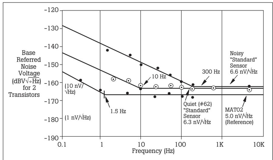
Figure 2. Base referred voltage noise: original sensor.
