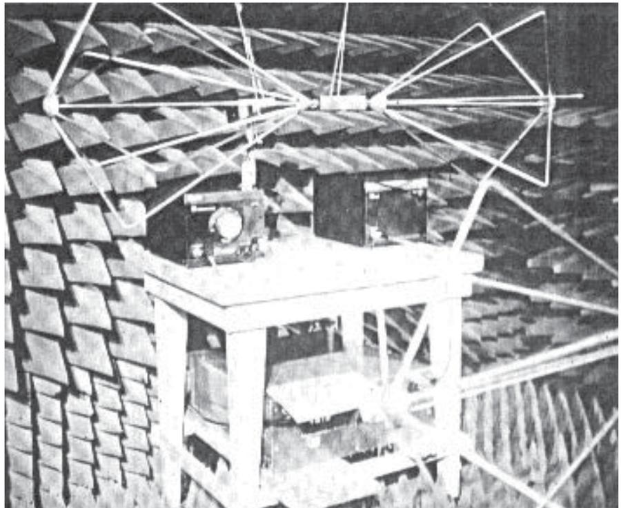
Figure 13. Electromagnetic interference immunity test setup.
