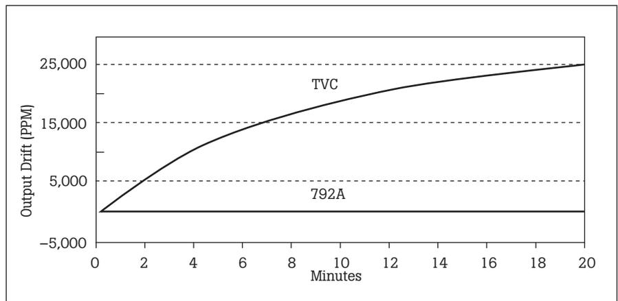
Figure 11. Output drift and stability 1000 V range.
