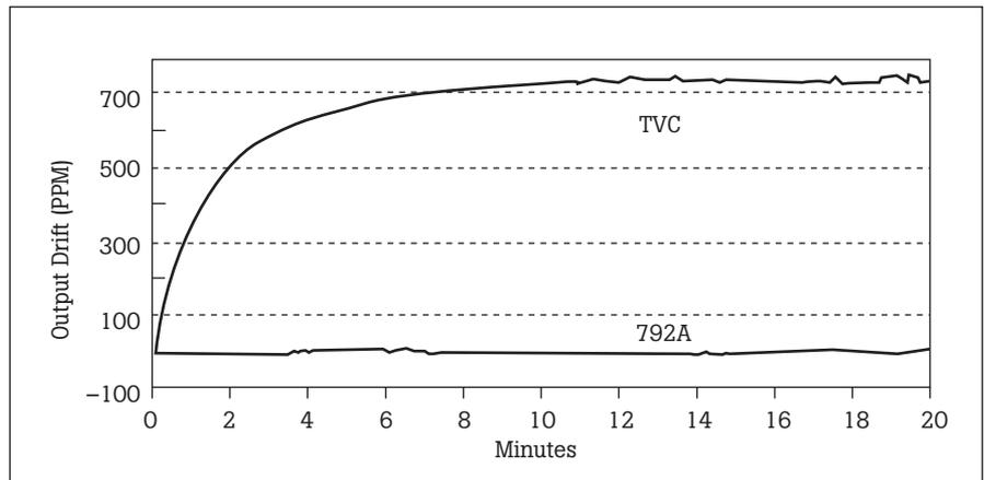
Figure 10. 792A output drift and stability 2 V range.
