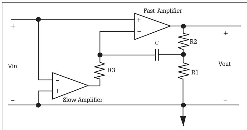
Figure 6. Noninverting composite amplifier.
