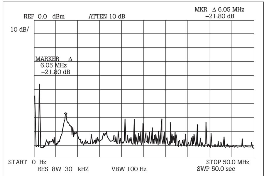
Figure 7. Spectrum of a calibrator output at 1 mV, 1 MHz.
