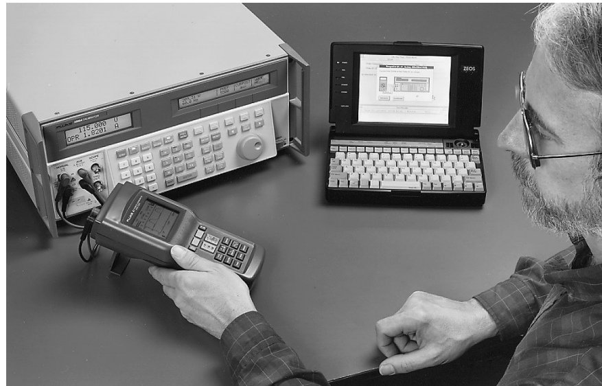
The Fluke 5500A Multi-Product Calibrator.
