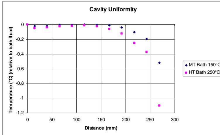
Figure 6. Temperature Uniformity of Cavity Walls.
