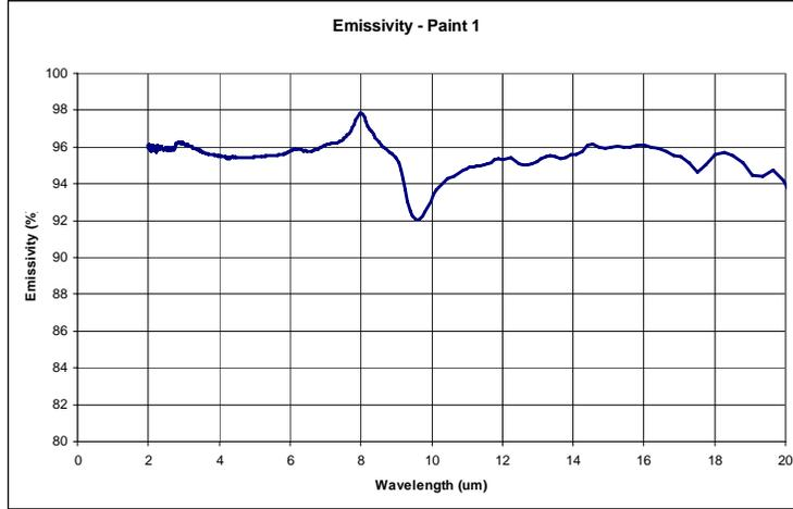
Figure 3. Spectral Response of 418X Emissivity.
