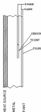
Figure 7. Heat Flow between Control Sensor and Target Surface.
