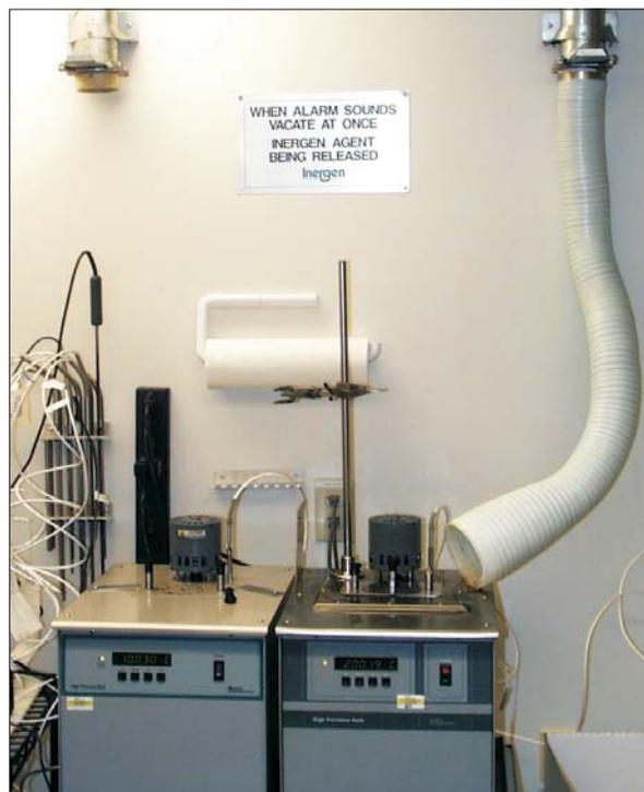
Figure 1 Ventilation system for removing oil vapors.
