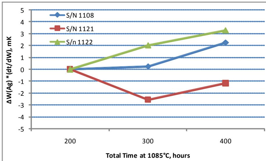
Fig. 6 Long-term stability at the freezing point of silver
