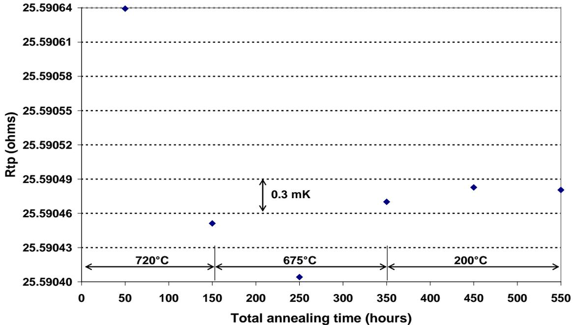
Fig. 4 Stability of an SPRT with partial oxygen pressure of 0.4 kPa
