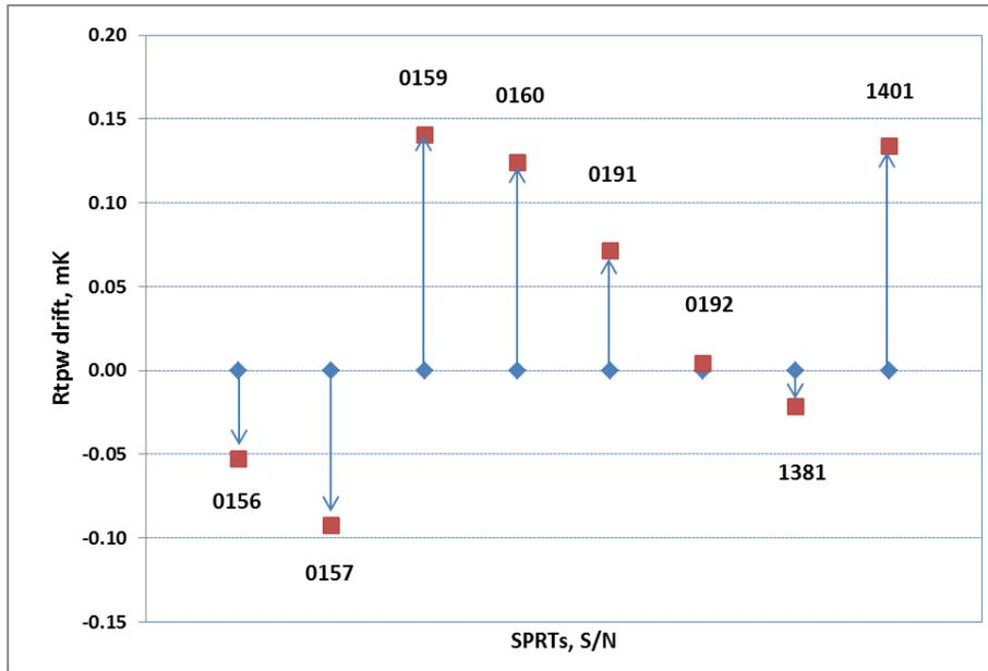
Fig. 2 Rtpw drift was evaluated after each of the eight SPRTs was held in LN<sub>2</sub> (-196 °C) for 100 hours
