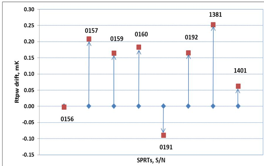
Fig. 3 Each of eight SPRTs was thermal cycled 10 times from LN<sub>2</sub> (held for 20 min) to 232 °C (stop at room temperature for 10 min)
