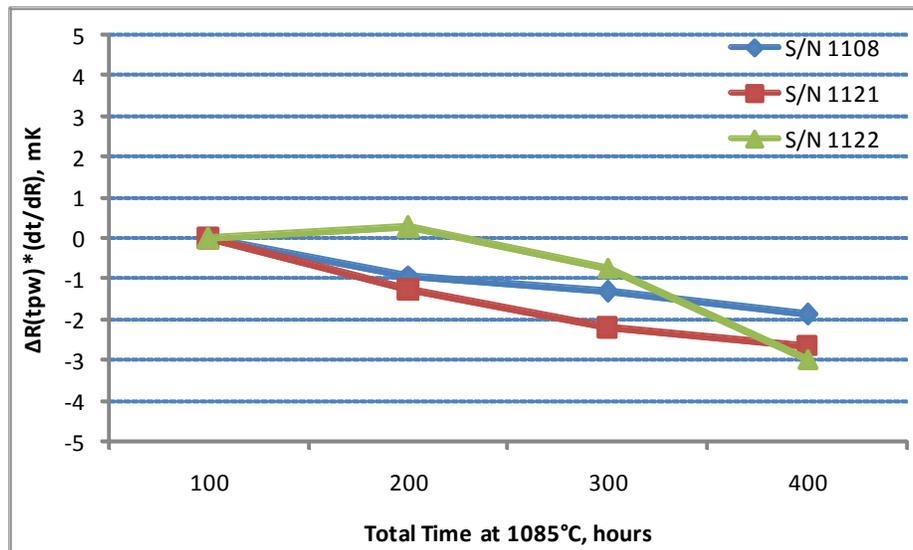
Fig. 5. Long-term stability at the triple point of water
