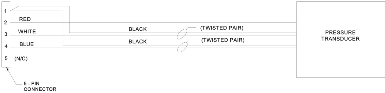
Figure 3: molbox1 and molbox1+ Components and Transducer Wiring Diagram
