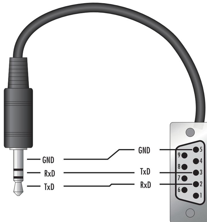
Figure 5. Serial Cable Wiring
