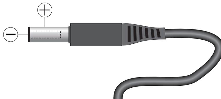
Figure 1. 12 V dc Power Source Polarity
