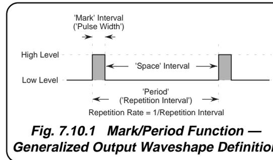
**Fig. 7.10.1 Mark/Period Function — Generalized Output Waveshape Definition**
