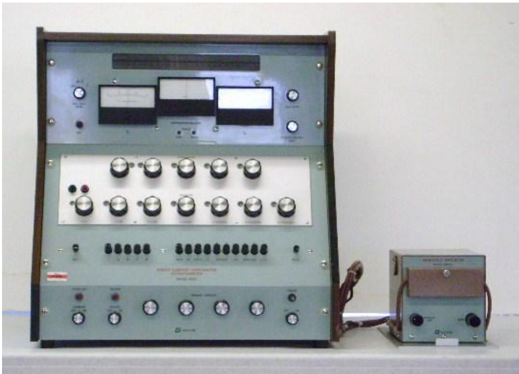
Figure 1. DCC Potentiometer with Light Beam Coupled Amplifier
