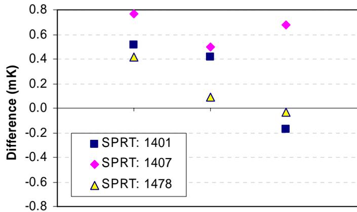
Fig. 4. Comparison between the short tin cell and standard size fused quartz glass shell tin cell.
