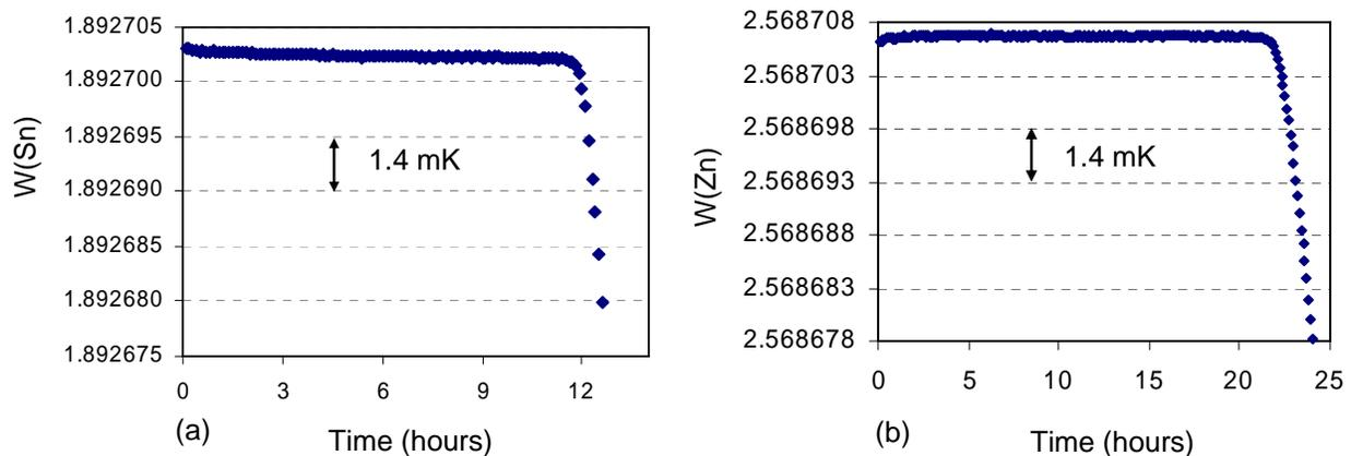
Fig. 3. Freezing plateau of the short tin cell (a) and the short zinc cell (b).
