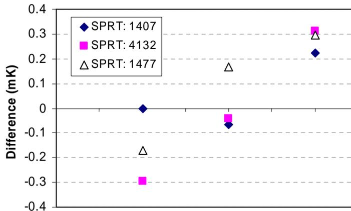
Fig. 5. Comparison between the short zinc cell and standard size fused quartz glass shell zinc cell.
