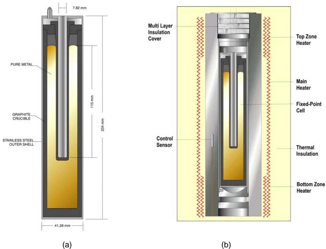
Fig. 1. Schematic drawing of the fixed-point cell (a) and the fixed-point system with the fixed-point cell and the maintenance furnace (b).
