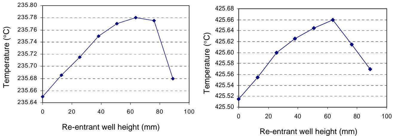
Fig. 2. Vertical temperature profiles of the tin and zinc cell furnaces.
