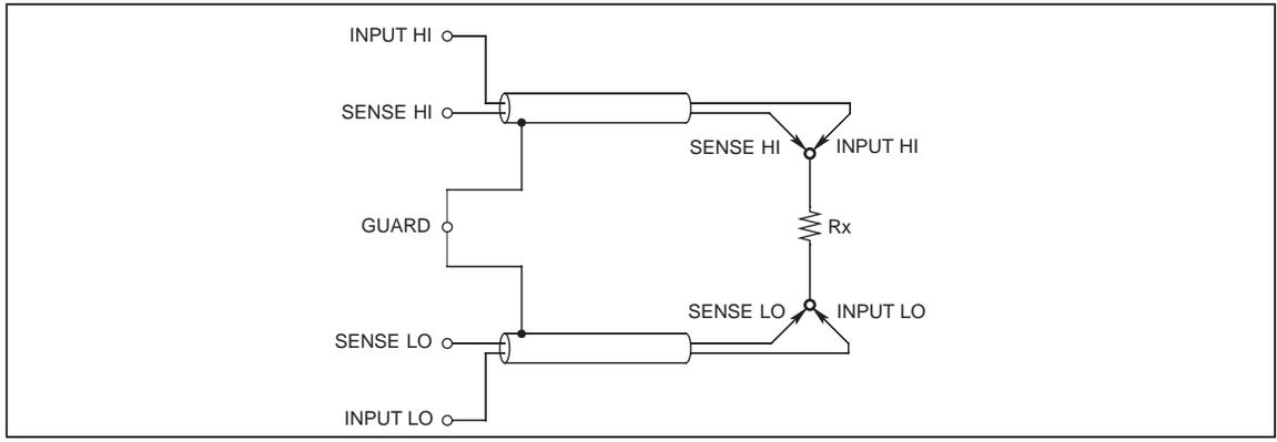
Figure 8. 4-Wire Measurements
