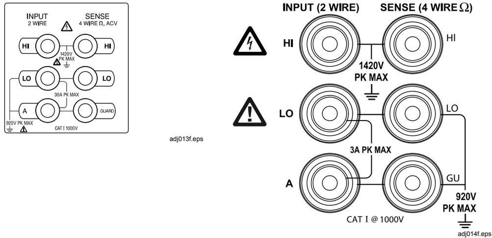
Figure 3. Front and Rear Input Terminals
