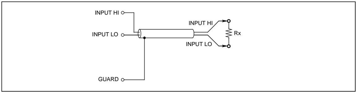
Figure 7. 2-Wire Measurements
