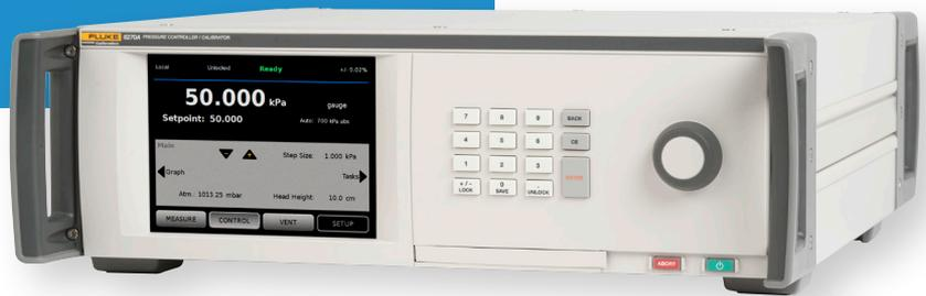
standards. Its measurement specification is typically cited to be as good as 0.005 % reading +0.005 % full scale. This specification includes the combined effects of non-linearity, hysteresis, and repeatability. It does not include long term stability, which is an additional 0.01 % reading per year. The specifications provided below for the Fluke Calibration 6270A include one-year measurement stability.
