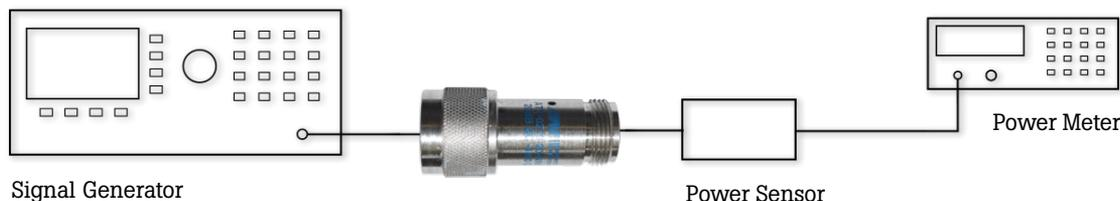
**Figure 1.** Using a 20 dB attenuator to reduce a signal source output level to within the power sensor input level range.
