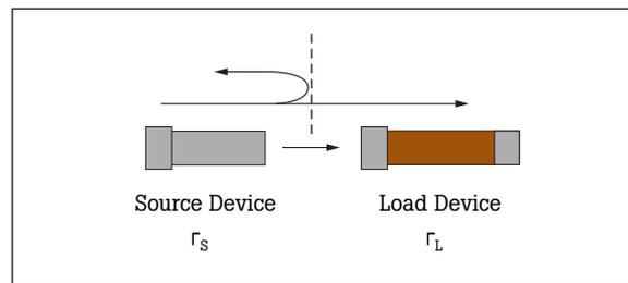
**Figure 1.** Reflection occurs at the mismatch between source and load.
