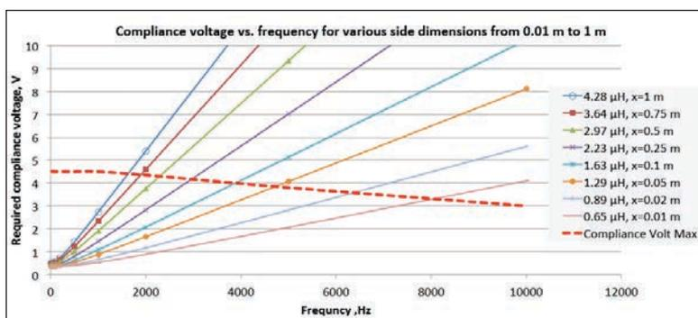
Figure 4. Required compliance vs. frequency for multiple loop widths.
