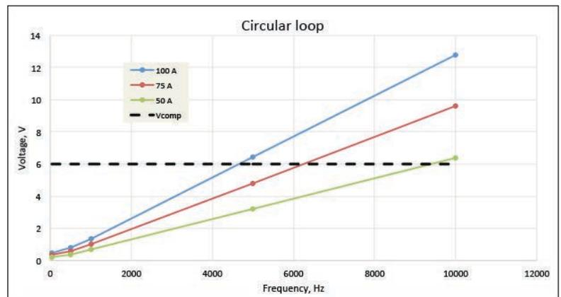
Figure 1. Determining the required compliance voltage. Selection of test setup is important.
