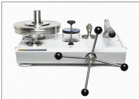
Performing a multi-dimensional calibration with a manually-operated deadweight tester like this one is a daunting task.
