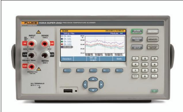
A temperature data logger such as this Fluke Calibration 1586A Super-DAQ can serve as the temperature reference, while also capturing measurements from the devices under test.
