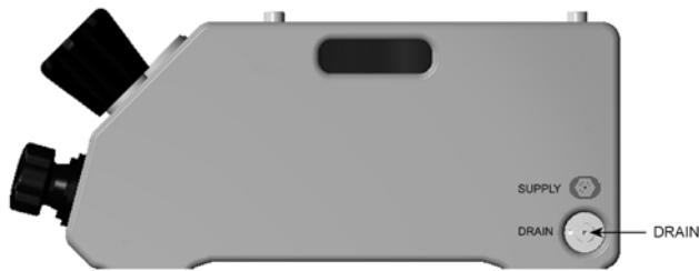
Figure 9. Drain Port Location
