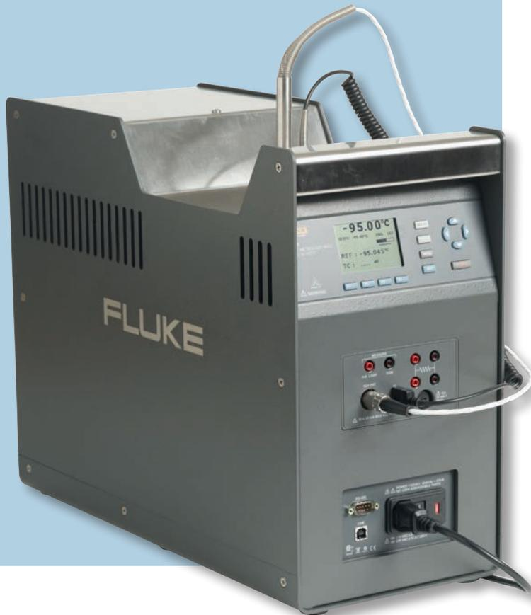
The 9190A Ultra-Cool Field Metrology Well provides excellent stability, uniformity and plenty of well depth for calibrating platinum resistance thermometers (PRTs), thermocouples, and other industrial thermometers. The 9190A offers  $\pm 0.2$  °C display accuracy over the full range. Applying the industry standard TUR of 4:1 allows you to achieve calibration accuracy of  $\pm 0.8$  °C using the dry-well display alone.
