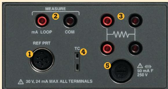
The **-P (process version) panel of the 9190A. Only available with -P configurations (e.g. 9190A-A-P).**
