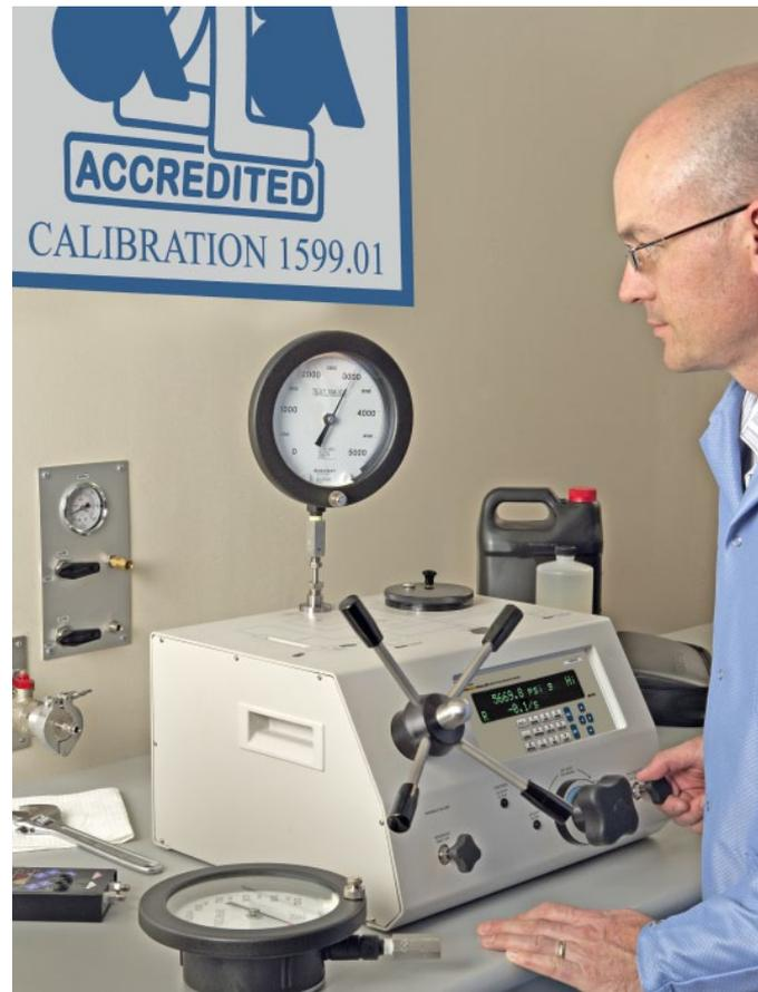
E-DWT-H’s fine adjustment valve enables the operator to set pressure to the exact nominal value on the gauge under test.
