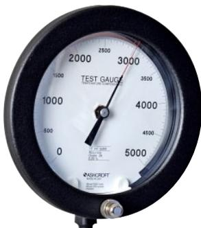
**Figure 1.** High pressure instruments such as the analog gauge pictured here are often calibrated using hydraulic test media.
