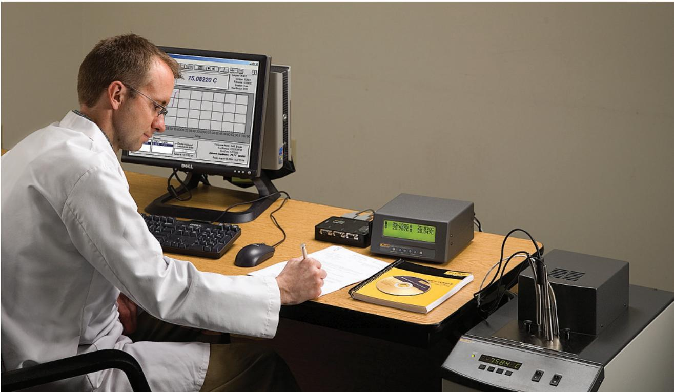
Why spend more time than necessary to calibrate PRTs, thermistors, and thermocouples? With a 7380 automated temperature calibration system from Fluke Calibration, you can perform consistent, repeatable calibrations quickly and efficiently. When the calibration is complete, you simply print out the report. It's that easy.
