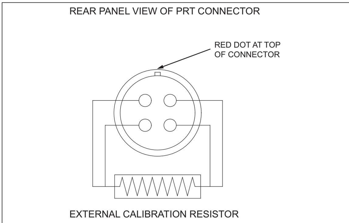
**Figure 1. Rear Panel PRT Connector - Temperature Circuit Calibration**
