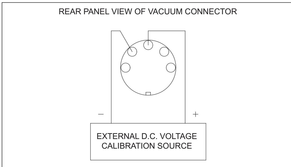
**Figure 2. Rear Panel Vacuum Connector - Vacuum Circuit Calibration**
