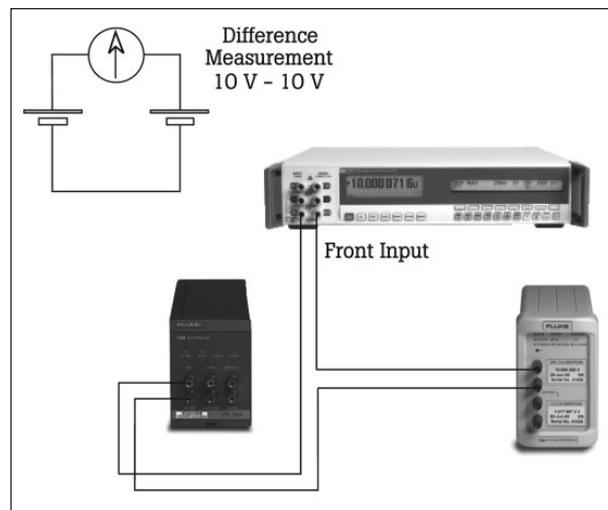
Fig. 2 The basic arrangement for comparing two standards at the 10 V level.
