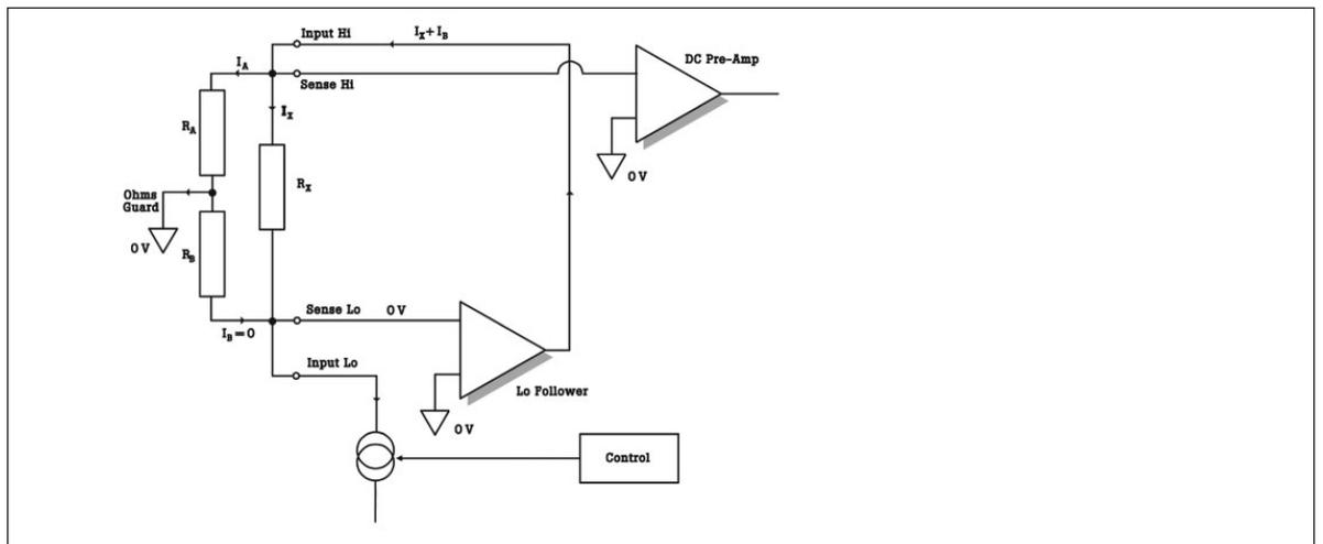
Fig. 11 Voltage ratio (resistance).
