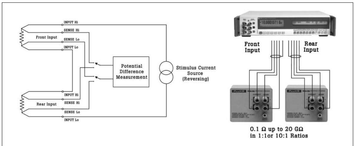
Fig. 10 True Ohms ratio.
