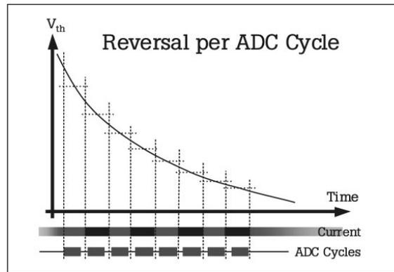
Fig. 6b Current reversal after each adc cycle.
