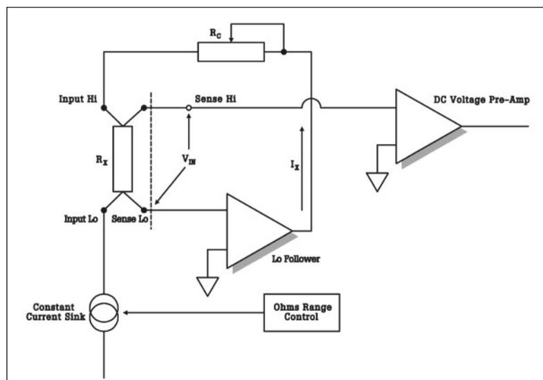
Fig. 4 Reference multimeter ohms converter.
