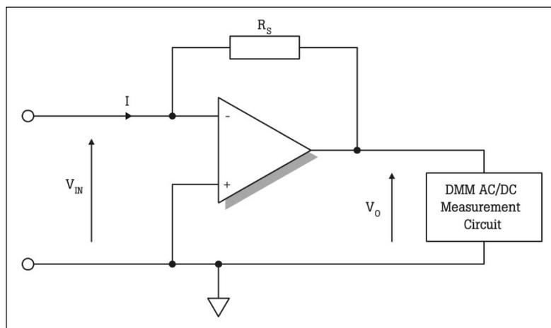
Fig. 14 Ammeter input ‘virtual earth’ current configuration.
