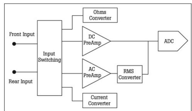
Fig. 1 Simplified DMM block diagram.
