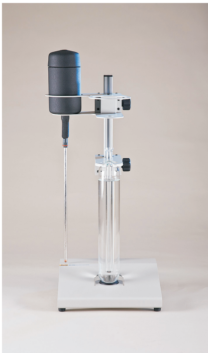
Figure 2 2031-STND with 2031A and triple point of water cell
