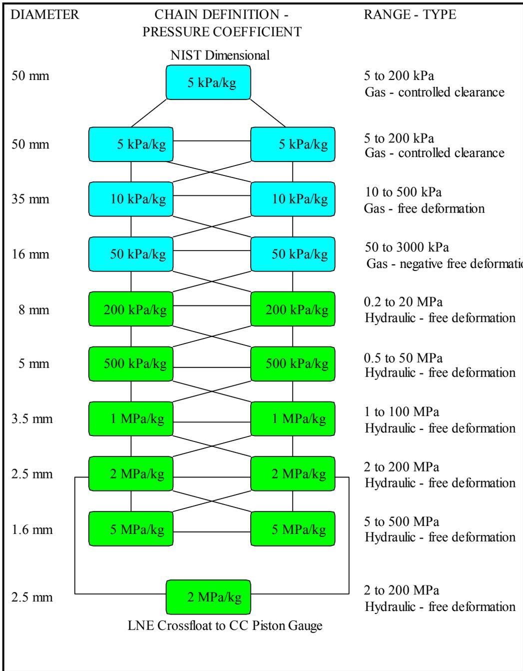
Figure 2. Structure of the 2001 piston-cylinder pressure calibration chain.
