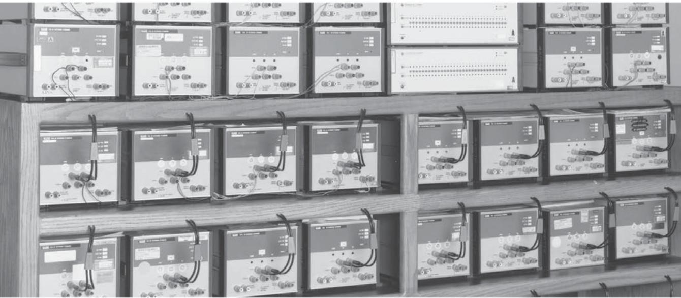
**Figure 3.** Several 732As and 732Bs support the Fluke Direct Voltage Maintenance Program with  $\pm 0.35$  ppm absolute uncertainty, traceable to NIST.
