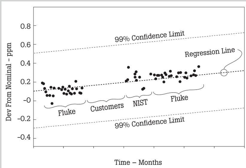
**Figure 6.** Calibration of a 732A transfer standard by NIST, as part of DVMP.
