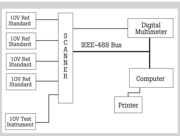
**Figure 4.** The Fluke Corporate Volt intercomparison system.
